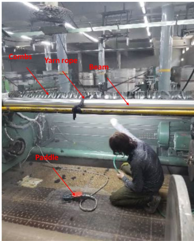
Fig.1. Re-beaming process setup
